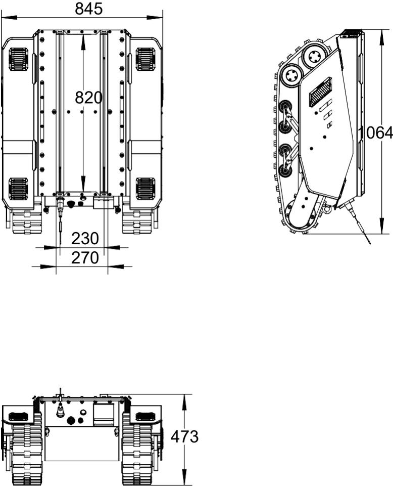
6.2 Illustration diagram of top extended support dimensions
